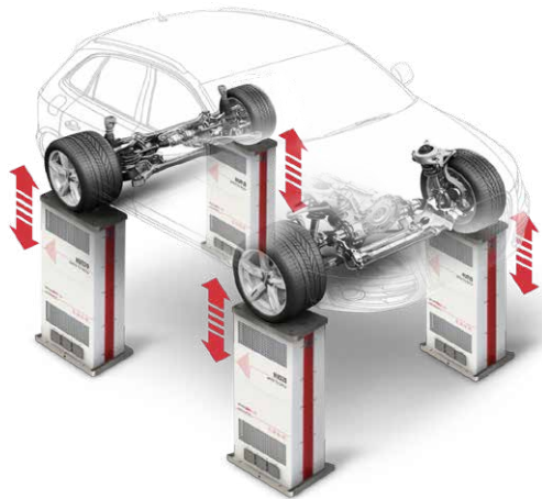
Shock absorber Test System HUD020 with 4 synchronized actuators
